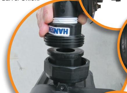
2. Connect new pipe to pipe by winding the Common Centre Nut onto the matching male thread
