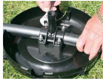
Select the Riser to suit your sprinkler size. Ensure fastening nuts are tightened evenly. Fit O-ring seal to sprinkler riser, locate riser spigot into hole in pipe and fasten the cross tee anchor.
