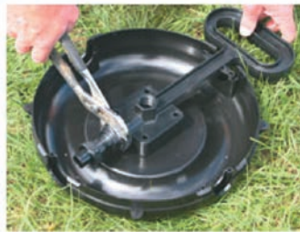
Screw on the Hansen Female Straight Coupler or the fitting to match your chosen hose/pipe to the end of the handle.
