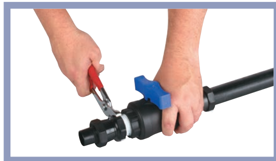
3. Do not over tighten. The recommended way to assemble a Ball Valve is finger tight. Tighten until firm with spanner or pipe grip. One to two turns should be all that is required.
