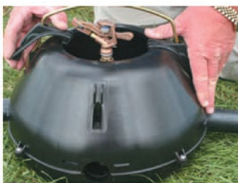
Fix wire clip into opposing holes on body sides. Ensure the wire runs parallel with the pipe as shown in the image.
