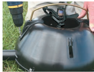
Fix wire clip into opposing holes on body sides. Ensure the wire runs parallel with the pipe as shown in the image. Screw wire clip holders into the holes provided.
