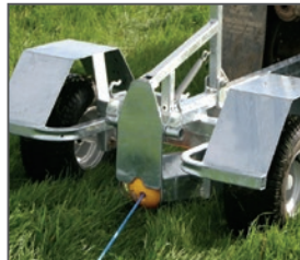
Step 4. Connect the Sub Main to the ATV via the Hansen™ Tow System; proceed to drag the Sub Main to the new location.
