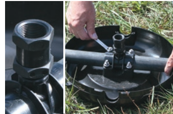
Fit O-ring seal to the under side of Riser. Screw the 20mm Hansen Socket onto the Riser thread and locate riser spigot into hole in pipe. Tighten nuts evenly to fasten the cross tee anchor and tighten socket.
