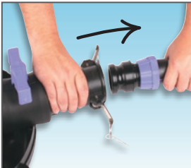
Step 3a Disconnect the Sub Main from the Drag Hose.
