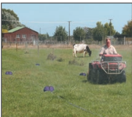
Step 5. Connect the Pod Sprinkler Lines to the ATV via the Hansen™ Tow System; proceed to drag the Pod Sprinkler Lines to the new location.
