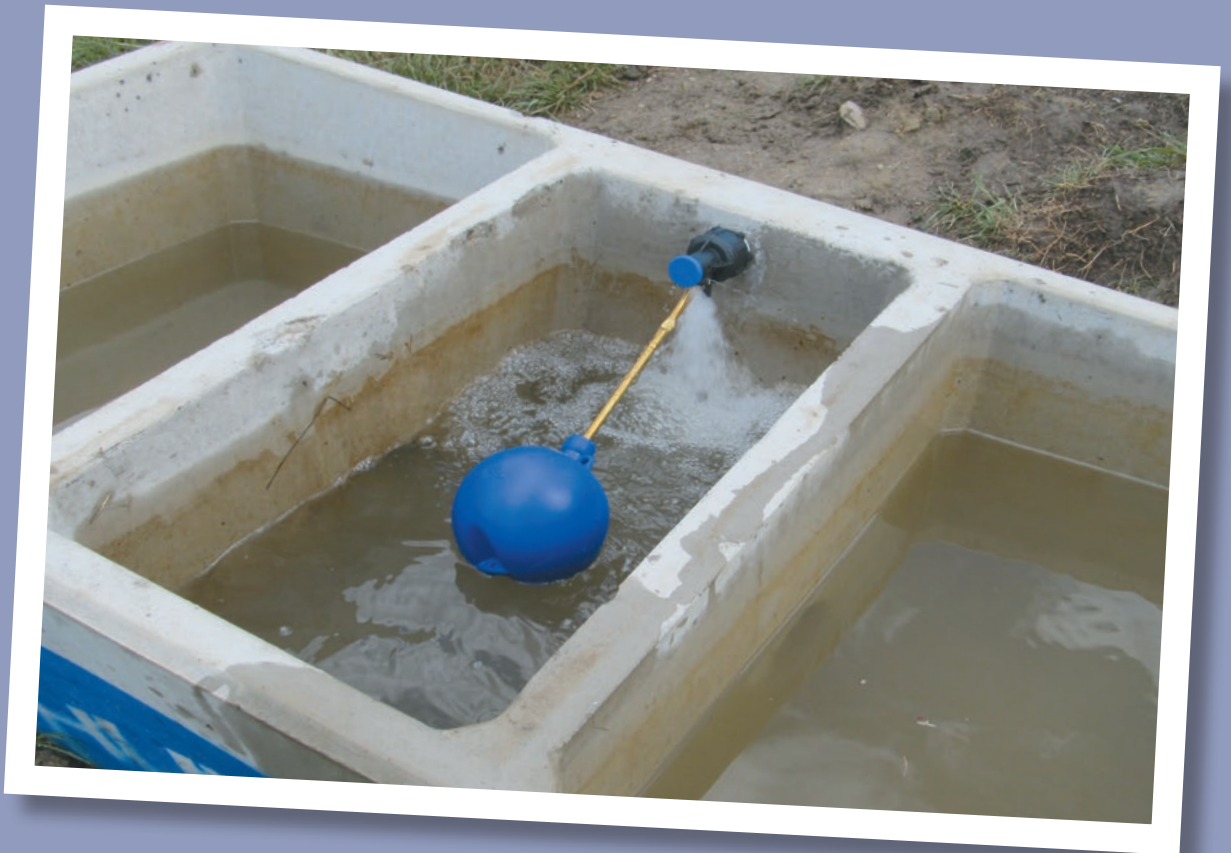
Hansen Fastflo Valve (HFFSV) in use
