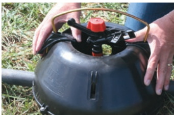
Fix wire clip into opposing holes on body sides. Ensure the wire runs parallel with the pipe as shown in the image.
