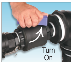
Step 8. Re-connect the Drag Hose to the Adaptor Set and turn on the Isolating Valve to begin irrigating at the new location.
